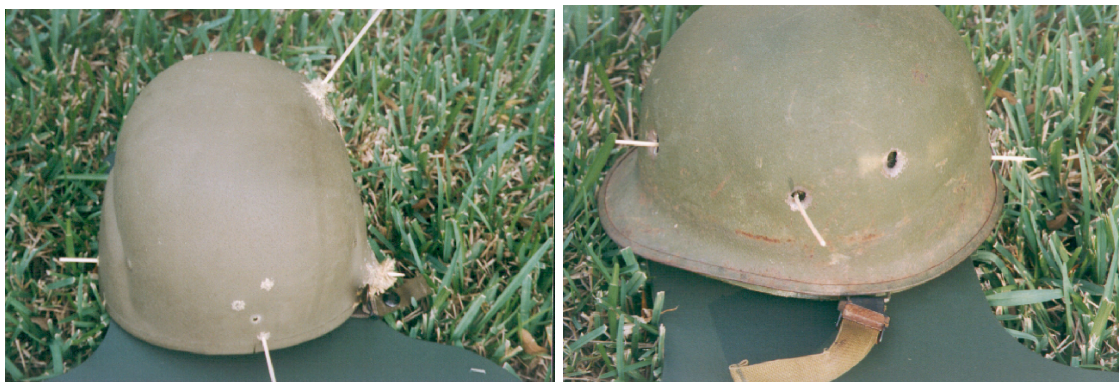
The 5.56mm MARS 55g FMJ completely penetrated both sides of the PASGT at 300 meters and one side of the M1 steel helmet with liner at 400 meters. Penetrating the M1 Helmet is the criteria used to establish the maximum effective range of small arms.
